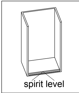
1. Ensure that the floor tray is level before you begin with the installation.
