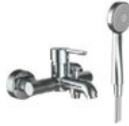
LUA H311081xxx1311 Bath mixer, fittings distance 134-166 mm, with fittings, synthetic flexible hose 1600mm and hand shower
